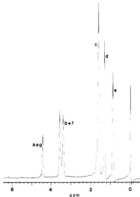
Figure 6. ^1\text{H} NMR spectrum of poly(0.75 2-Bu-DOP-co-0.25 DOL).
